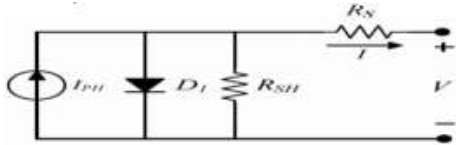
Fig.1: The equivalent circuit of a PV cell.
