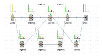
Fig. 8: Parallel or Mixed Transfer Line for Multiple Operation with Bottleneck Analysis and Multiple Single Process
