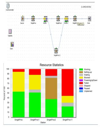
Fig. 7: Parallel or Mixed Transfer Line for Multiple Operation with Multiple Buffer and experimental setup
