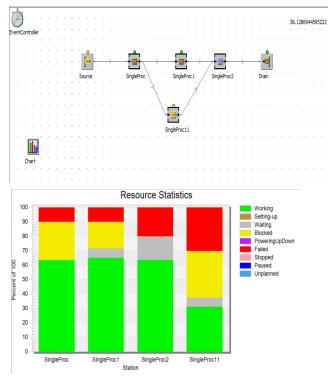
Fig. 3: Graph on Parallel or Mixed Transfer Line for Multiple Operation
