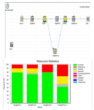
Fig. 5: Parallel or Mixed Transfer Line for Multiple Operation with Multiple Buffer
