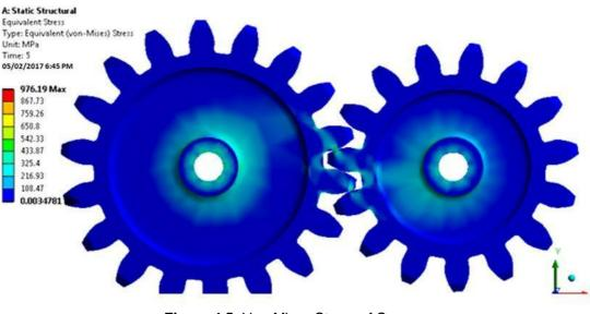
Figure 4.5: Von-Mises Stress of Spur gears
