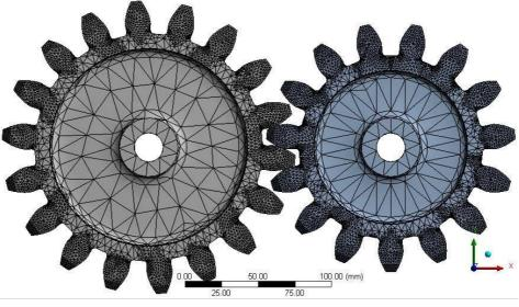
Figure 3: Meshed model of spur gear
