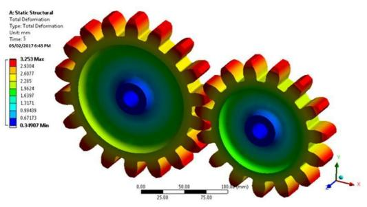
**Figure 4.5:** Total Deformation of Spur gears The maximum and minimum total deformation values found are 3.253mm and 0.34907 mm.
