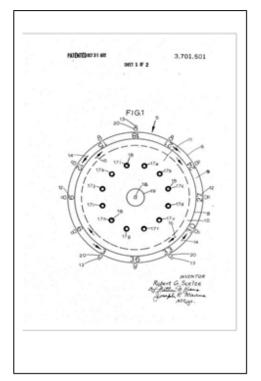
**Figure 2.** Old circular airport design: (a) Airport design by James S. Conrey, US Patent 3157374, 1964 [6], and (b) Two Circular Runways design by Robert G. Scelze, US Patent 3701501, Oct 1972 [7]
