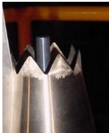
Figure 1. Chevron exhaust engine designed to reduce jet noise [11]
