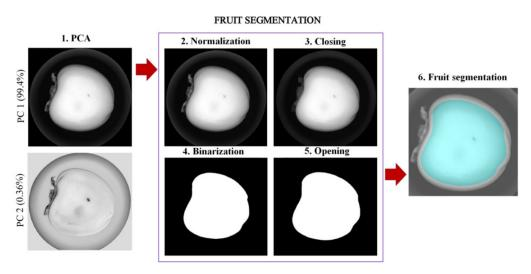
Figure 3. Steps performed for background, calyx and fruit segmentation.
