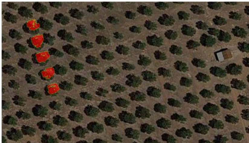
Figure 4. Projection of the 3D scanned points superimposed on a Google satellite view of the field.
