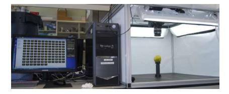
Figure 1 - Image capturing computer vision system
