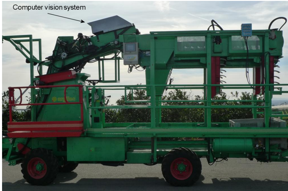
338 339 Figure 8. Mobile platform with the grading system
