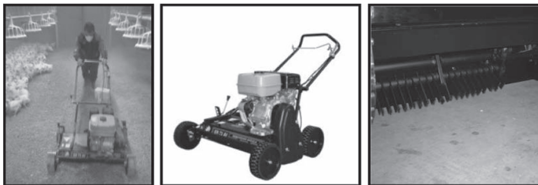
Figure 1. Machine used for litter aeration (LA) and detail of the rotative parts.
