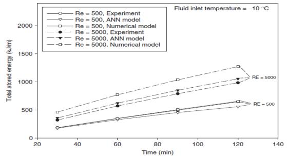
Figure 7. Variation of total stored thermal energy with time, using the ANN approach, the numerical model, and experimental data, for Re = 500 and 5000 and a HTF inlet temperature of  $-10 \circ C$  [35]
