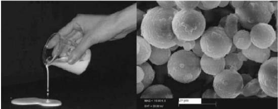
Figure 6. Flowing microencapsulated PCM as a phase-change slurry [29]
