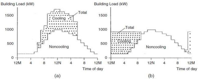
Figure 2. Daily load profiles of a building energy load: (a) no storage and (b) full storage [18]
