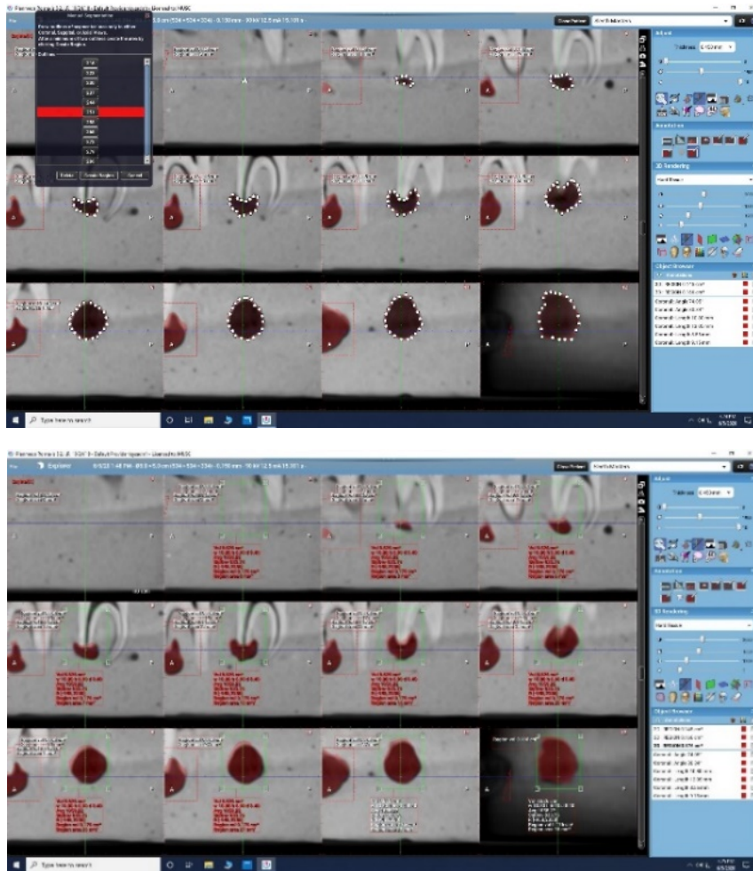
Figure 4: Romexis free region grow tool used to calculate osteotomy volume. The image on the top shows the outlines of the region being identified in successive 1mm planes. The image on the bottom shows the data output once the outlines were completed.
