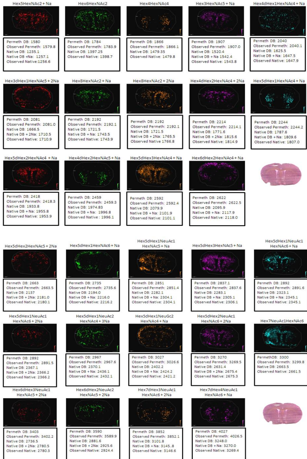
Figure 13. Mouse Brain N-Glycan Imaging Panel. 28 N-glycans were observed in both the MALDI-IMS dataset and the permethylation spectra. These ions vary with respect to brain histology.
