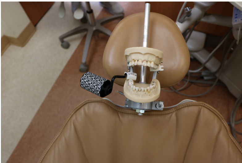
Figure 4. Dentoform mounted to dental operatory chair with attached X-Clip (containing the fiducials) and patient tracker.
