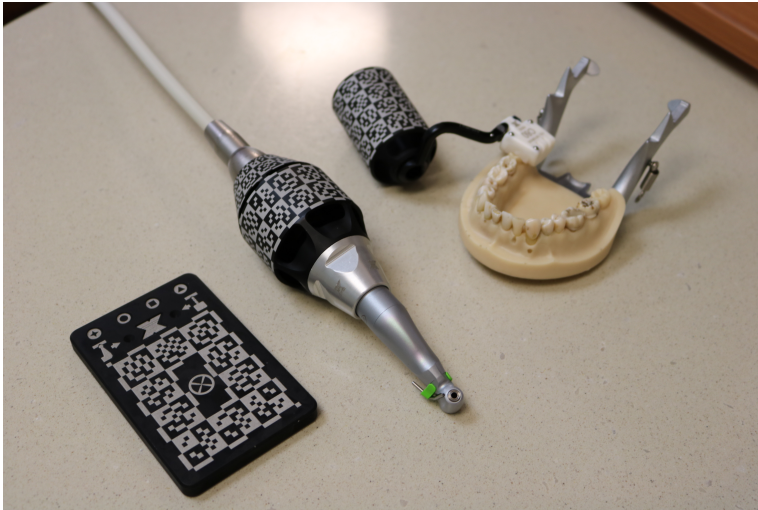
Figure 7. Image displaying the Go-plate, Surgical Handpiece and X-Clip with fiducials and attached patient tracker.
