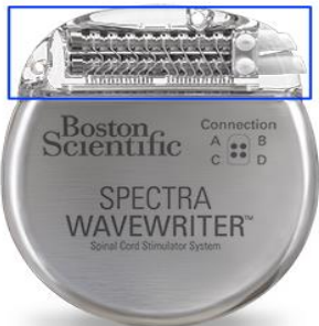
Figure 6: Image modified from [22]. Image of Spectra WaveWriter IPG manufactured by Boston Scientific (Marlborough, MA). Blue box highlights the connection ports for the stimulator paddle.
