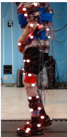
Figure 17: Subject fitted with LED markers during walking task.
