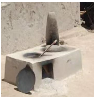
Dimensions: Length 32 inches, width 16 inches, Height 10 inches Baffle height 5 inches, Chimney diameter 4 inches
