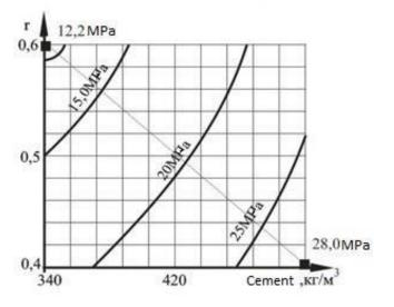
Fig. 1. Influence of composition factors on cube strength where r - aggregate-Structural factor; LI3 - cement-ash binder
