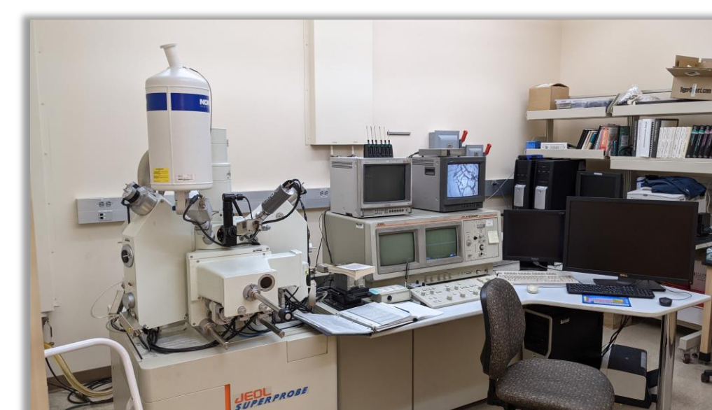
Fig. 4 JXA-8900R Electron Probe Microanalyzer (Jeol, USA)
