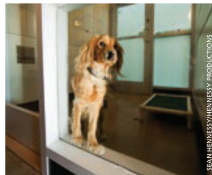
The Potter League houses its dogs in individual, indoor/outdoor rooms that use laminated glass (both clear and translucent panels) in anodized aluminum frames and a sprayed acoustical plaster on the walls to control noise.
