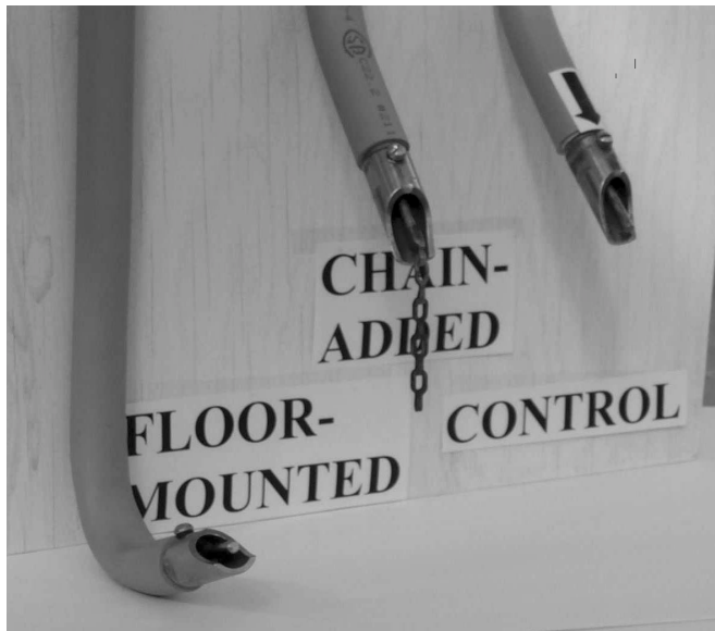
Fig. 1. From left to right, the floor-mounted, chain-added and control nipples. A continuous drip adjustment screw was installed on all nipples to allow the continuous drip feature to be used as required (arrow on 'CONTROL' nozzle shows screw location).
