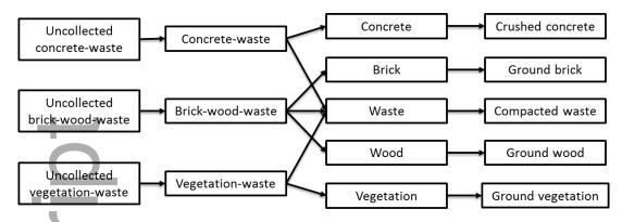
Figure 4 – Debris types considered in the case study
