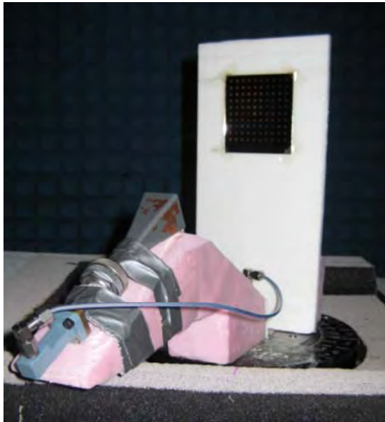
Fig. 5. The measurement setup of the reconfigurable reflectarray.
