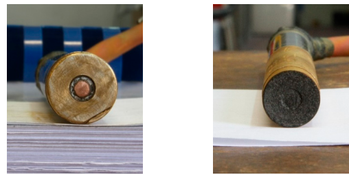
(b) Carbonaceous matter on (not cooled) heat flux probes (black soot).
