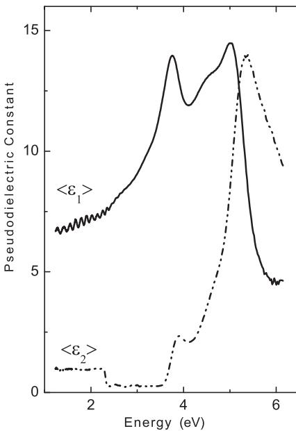
Fig. 5. Spectral dependence of the pseudodielectric function for  $\text{Ga}_2\text{SeS}$  crystals. Solid and dot-dashed curves represent the real and imaginary part spectra, respectively.
