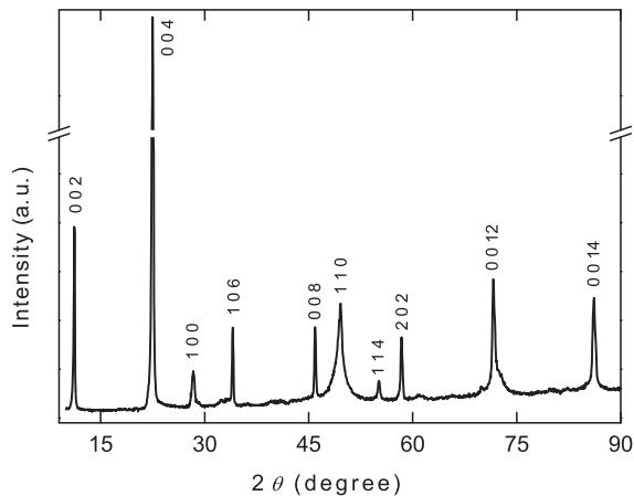
Fig. 2. X-ray powder diffraction pattern of  $\text{Ga}_2\text{SeS}$  crystal.
