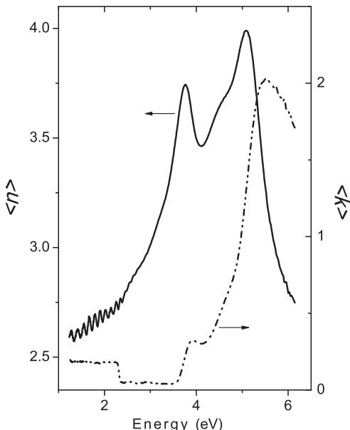
Fig. 6. Spectral dependence of the pseudorefractive index and pseudoextinction coefficient for  $\text{Ga}_2\text{SeS}$  crystals.
