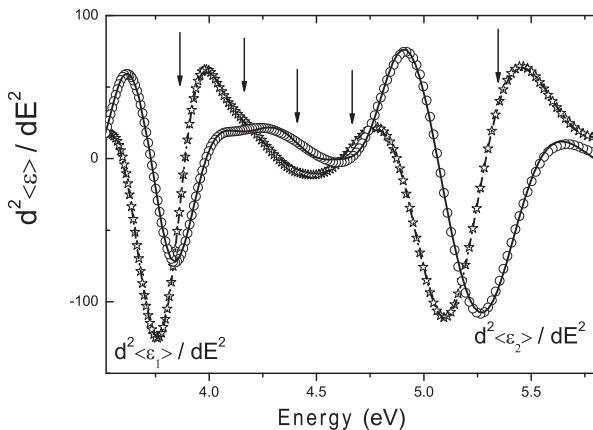
Fig. 7. Second-energy derivative spectra of the pseudodielectric function for  $\text{Ga}_2\text{SeS}$  crystals. Stars and open circles represent the second derivative spectra of the real and imaginary parts of the pseudodielectric function, respectively. The solid and dot-dashed curves show the fit to the experimental data.
