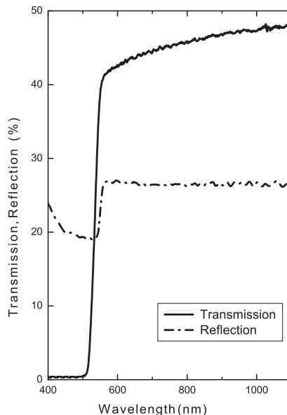
Fig. 3. The spectral dependence of transmission and reflection at room temperature for  $\text{Ga}_2\text{SeS}$  crystal.
