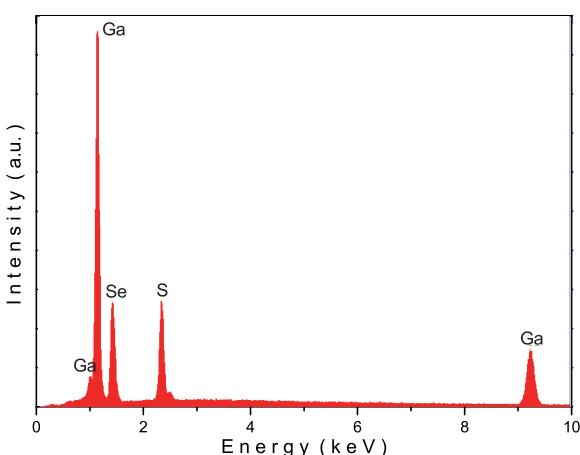
Fig. 1. Energy dispersive spectroscopic analysis of  $\text{Ga}_2\text{SeS}$  crystal.
