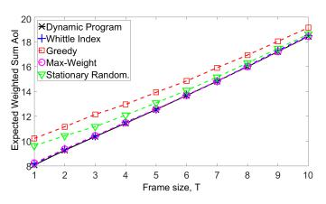
Fig. 6. Two-user general network with  $K = 200, \alpha_i = 1, p_1 = 2/3, p_2 = 1/10, \forall i$ . The simulation result for each policy and for each value of *T* is an average over 1,000 runs.
