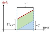
Fig. 3. Area under  $AoI_i$  during any frame k in terms of  $h_{k,i}$  and T.
