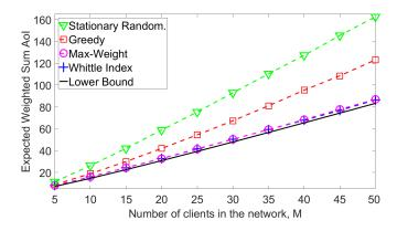
Fig. 7. Network with  $T = 2, K = 50,000, \alpha_i = 1, p_i = i/M, \forall i$ . The simulation result for each policy and for each value of *M* is an average over 10 runs.
