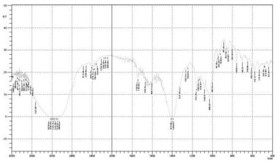
**Figure 4.4** FTIR spectrum of levocetirizine- $\beta$ -CD complex.
