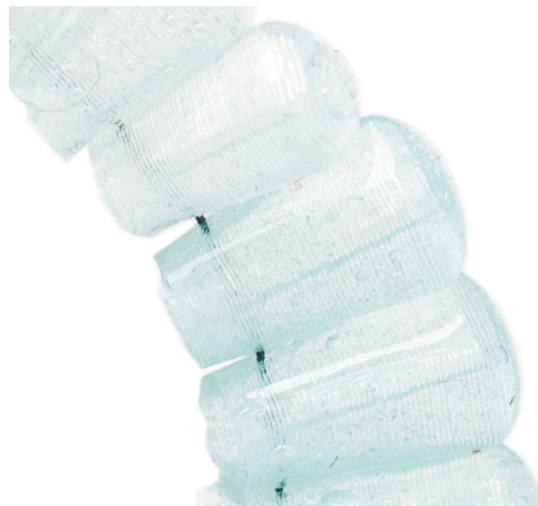
Figure 6 | After sifting the pigment prior to use through a 120 mesh sieve, the speckles have disappeared, leaving only the pure pigment behind.
