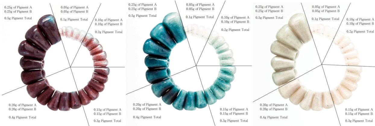
Figure 4 | An example of a reverse colour change with low-temperature powdered leuco pigments. Both pigments (Turquoise 22°C and Orange 19°C) appear as pastel colours at room temperature (far right sample). Full colour saturation (left sample) occurs at around 5°C.
