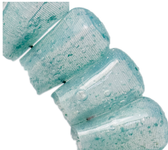
Figure 5 | Large Pigment speckles are clearly visible in the silicone shapes made with unsifted powdered Leuco pigment.
