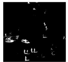
Figure 8 | OpenCV library example of background subtraction
