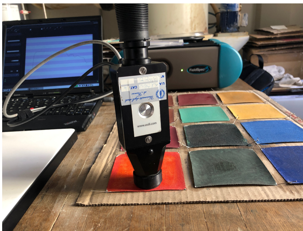
Figure 1 - Portable hyperspectral sensor, ASD FieldSpec FR Pro 3.
