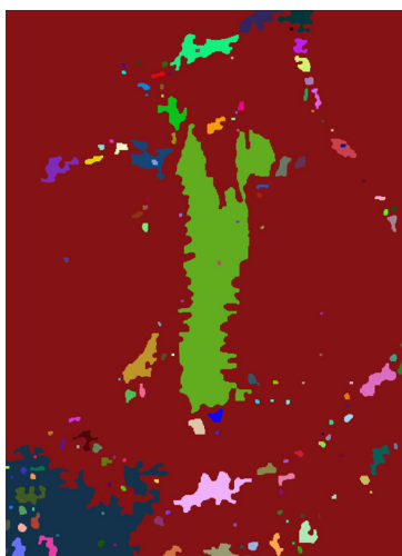
figure 7 - Result of region group: each identified region is displayed with a different colour.
