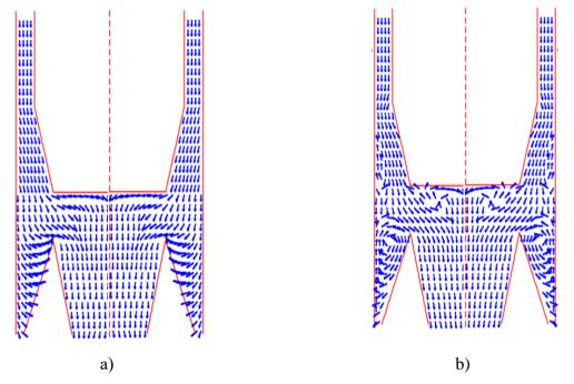
**Fig. 5.** a- using the vorticity and the current function, b- A semi-implicit method for pressure binding SIMPLE.
