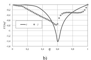
**Fig.4.** Profiles, a) axial, b) radial and c) tangential air flow velocities in cross section  $\xi$  =0.7 at *Wref* /*Uref* =1. 1- using vorticity and current function, 2- Semi-implicit method for pressure coupling SIMPLE.
