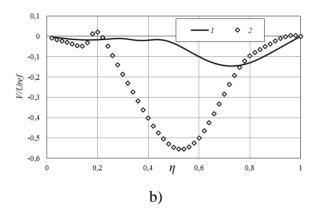
**Fig.3.** Profiles, a) axial, b) radial and c) tangential air flow velocities in cross section  $\xi$  =0.65 at *Wref* /*Uref* =1. 1- using vorticity and current function, 2- Semi-implicit method for pressure coupling SIMPLE.
