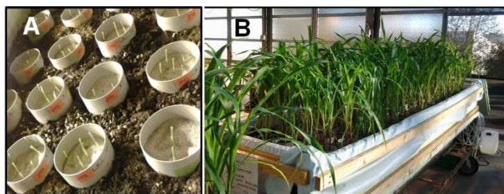
Chapter 2. Suppl. Fig. 1. Cooling system for adjustment of low root zone temperature based on moist peat culture substrate with cooling tubes. A) Pots with germinating maize seedlings inserted into the cooling system. B) Overview at final harvest.
