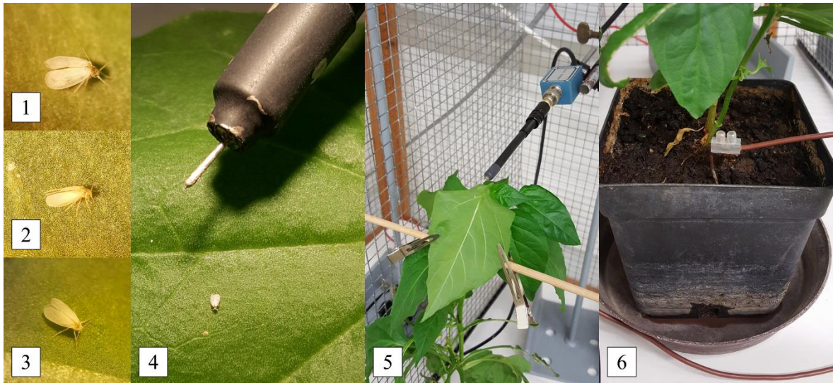
Figure 6: Experimental setup of the EPG system
