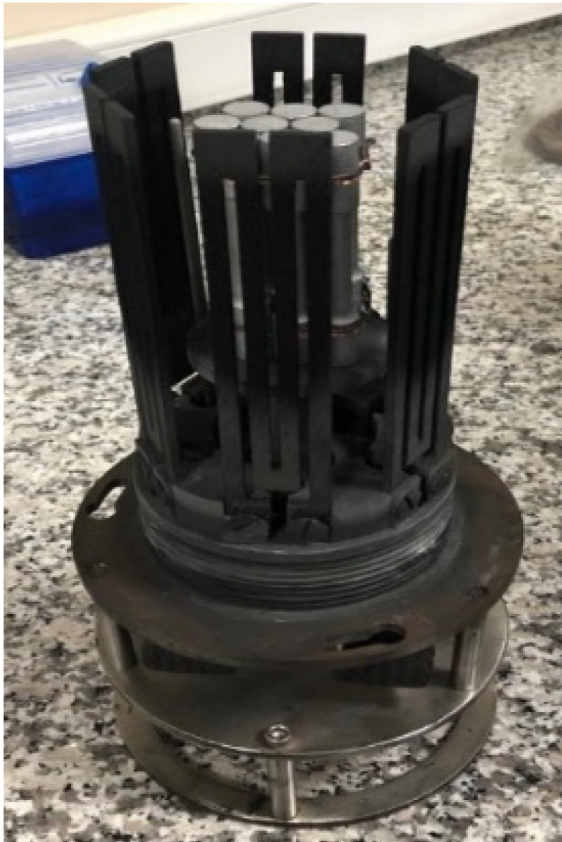
Figure 1 Graphite heating setup with a set of samples
