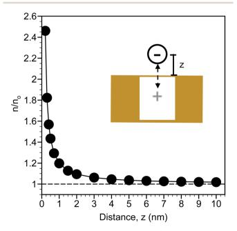
Fig. 2 Calculated monovalent ion distribution (n, normalized relative to the bulk concentration as  $n/n_{\rm o}$ ) extending from a planar gold surface arising from "image charge", depicted in the schematic. The variable z represents the distance from the surface to the center of the ion.
