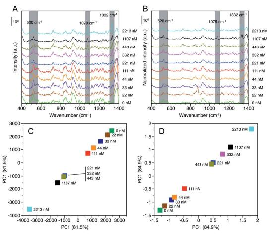
Fig. 3 SERS spectra of nitrate based on (A) intensity (baselined) and (B) normalized intensity (baselined + SNV). Greyed regions at 1079 cm<sup>-1</sup> and  $1332 \text{ cm}^{-1}$  denote NO<sub>3</sub><sup>-</sup> peaks used for adsorption analysis and the region at 520 cm<sup>-1</sup> denotes the silicon peak from the SERS substrate. PC1 plots corresponding for (C) baselined and (D) normalized time-averaged spectra over the range 1000 cm<sup>-1</sup> to 1350 cm<sup>-1</sup>
