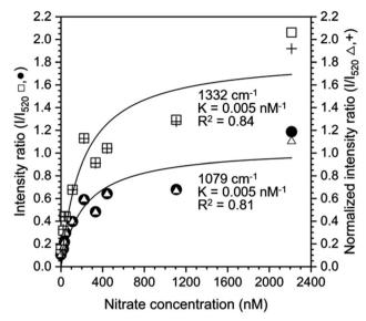
Fig. 5 Intensity and normalized intensity ratios ( $I/I_{520}$ ) based on the silicon peak at 520 cm<sup>-1</sup> and nitrate peaks at 1079 cm<sup>-1</sup> (closed circles  $\bullet$ , open triangles  $\triangle$ ) and 1332 cm<sup>-1</sup> (open squares  $\square$ , plus signs +) as a function of nitrate concentration. The solid lines show the fitted Langmuir adsorption model and the Langmuir constant K and the goodness of fit,  $R^2$ , are reported.
