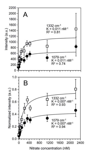
Fig. 4 (A) Intensity and (B) normalized intensity of the peaks at 1079 cm $^{-1}$  (closed circles  $\bullet$ ) and 1332 cm $^{-1}$  (open squares  $\square$ ) as a function of nitrate concentration. Error bars represent the time-averaged standard deviation of the intensities at the specified wavenumbers. The solid lines show the fitted Langmuir adsorption model and the Langmuir constant K and the goodness of fit,  $R^2$ , are reported.
