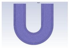
Figure 31:Polyhedral Mesh of Fluid for fine refinement test case with prism layers on Fluid-Pipe-Interface
