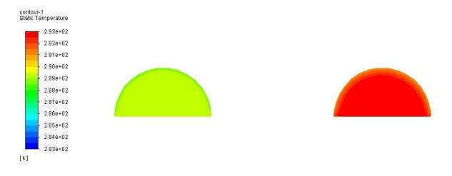
Figure 56: Inlet and Outlet Temperature Contour
