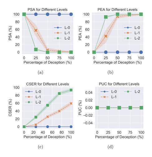
Figure 8.2: Performance evaluation of seed-based DDAF for different levels of FDI attacks, where a) PSA decreases, b) PEA increases, c) CSER increases, and d) PUC remains the same with increasing randomized sensors.
