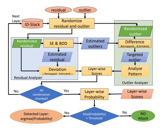
Figure 6.3: Block diagram for attack detection and localization.
