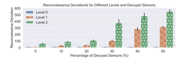
Figure 8.1: Impacts of decoy data on reconnaissance deviation for different levels. Reconnaissance deviation increases as more sensors are used to add decoy data supporting the ID randomization. A higher level considers more sensors in the node; thus, the decoy data become more effective.
