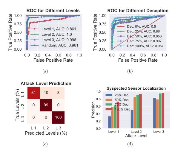
Figure 8.4: Performance evaluation of seed-based DDAF on attack detection, and localization for different levels of FDI attacks. a-b) attack detection, c) attack levels, and d) suspected sensors.
