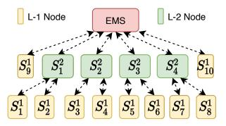
Figure 2.2: Tree diagram of a two-level hierarchical communication network.
