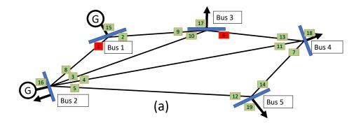
Figure 6.6: Distribution of the suspected sensors 1, and 6 for an FDI attack at Level 1, which indicates a lower probability of attack.
