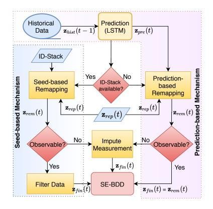
Figure 6.14: Hybrid remapping mechanism.
