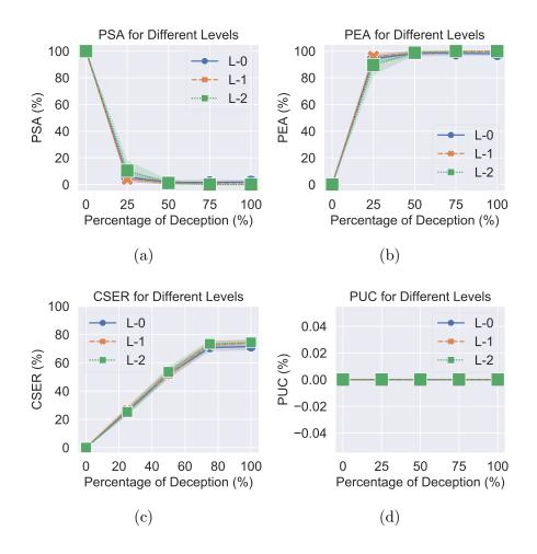
Figure 8.8: Performance evaluation of prediction-based DDAF for different levels of FDI attacks, where a) PSA decreases , b) PEA increases, c) CSER increases, and d) PUC remains the same with increasing randomized sensors.
