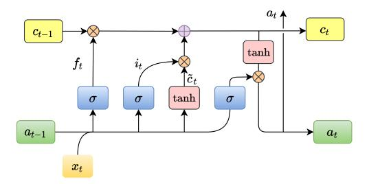
Figure 3.3: A block of LSTM architecture
