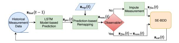
Figure 6.10: Prediction-based remapping mechanism.
