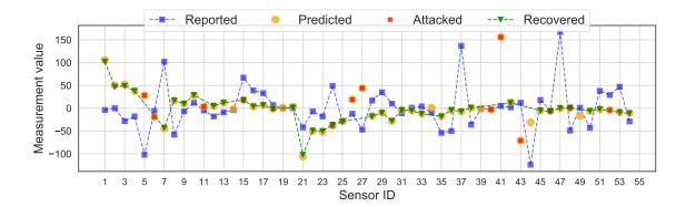
Figure 6.13: Prediction-based remapping mechanism under FDI attack, where the attacked sensors are omitted during the remapping and keeps the state estimation resilient to the FDI attacks.
