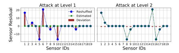
Figure 6.8: Residual estimation under an FDI attack. Level 1 shows high deviations in the residual estimation, presenting a lower chance of FDI attack. Whereas Level 2 shows almost zero deviations indicating a higher chance of FDI attack.
