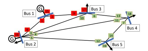
Figure 6.7: Distribution of the suspected sensors 1, 2, 8, 9, 15, 16, and 17 for an FDI attack at Level 2, which indicates a higher probability of attack.
