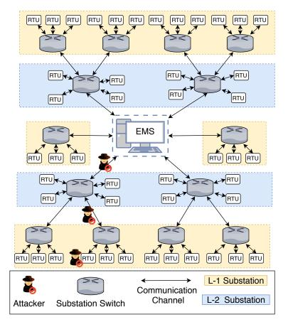
Figure 2.1: A two-level hierarchical communication network in power grids.
