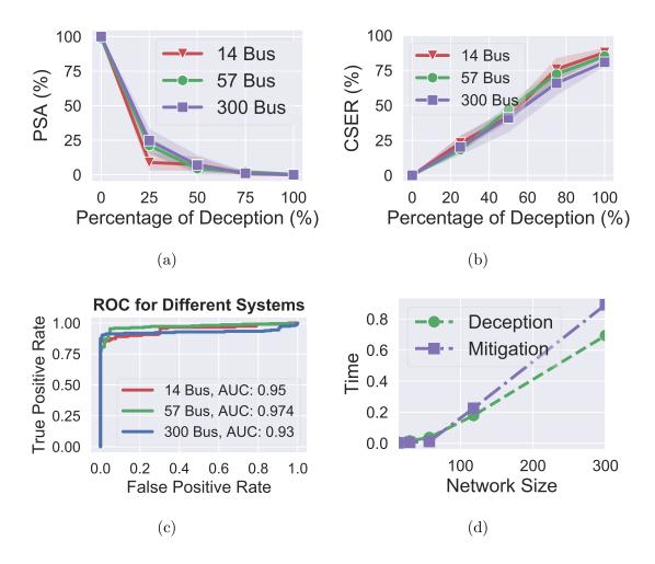
Figure 8.7: Scalability analysis of DDAF for different models. a) PSA, b) CSER c) attack detection, and d) running time (seconds) show DDAF is scalable for different test cases.
