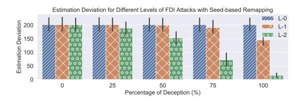
Figure 8.3: Estimation deviation of seed-based DDAF for different levels of FDI attacks, where a higher deception decreases the estimation deviation.
