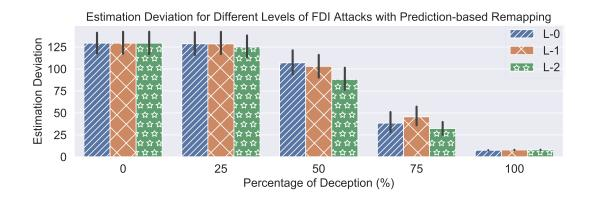
Figure 8.9: Estimation deviation of prediction-based DDAF for different levels of FDI attacks, where a higher deception and levels decrease the estimation deviation.
