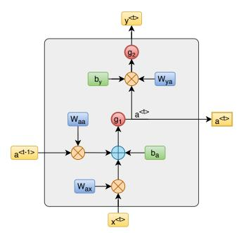
Figure 3.2: A block of RNN chain architecture
