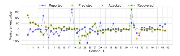
Figure 6.12: Prediction-based remapping mechanism under normal condition, where almost 91% (49 out of 54) of the randomized sensors are remapping accurately.
