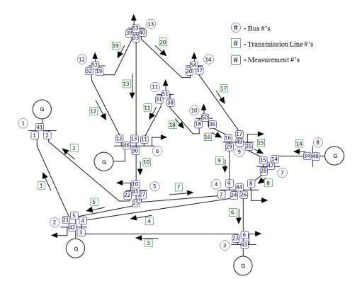
Figure 6.11: IEEE 14-bus test system [RASK14].
