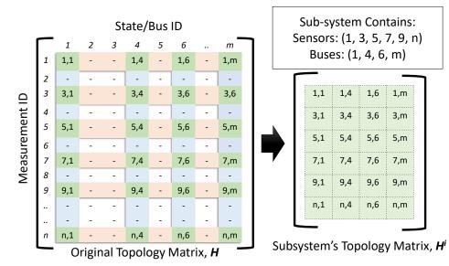
Figure 5.2: Generation of topology matrix of the subsystem.
