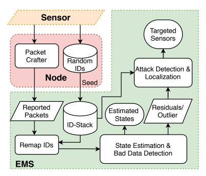
Figure 6.1: Block diagram of seed-based DDAF.
