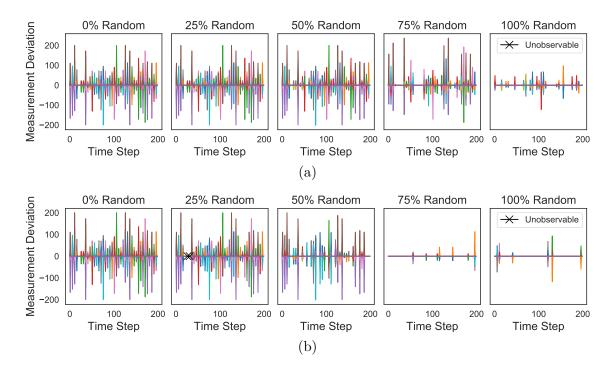
Figure 8.11: Measurement deviations for different sensors only with seed-based remapping under FDI attacks at a) Level 1, and b) Level 2.
