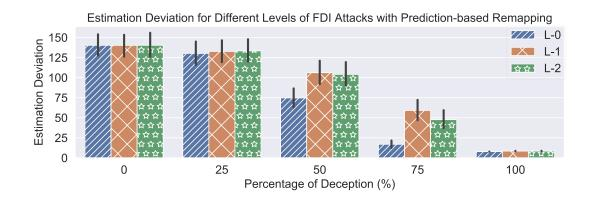
Figure 8.14: Estimation deviation of hybrid DDAF for different levels of FDI attacks, where a higher deception and levels decrease the estimation deviation.
