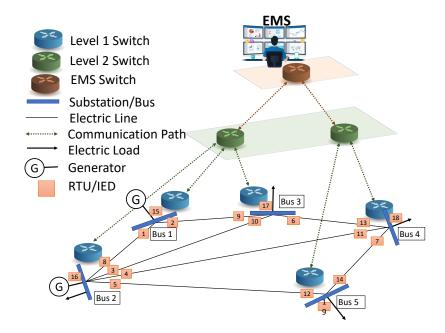
Figure 6.4: SCADA Network of IEEE 5 bus system.
