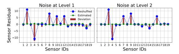
Figure 6.9: Residual estimation with random noise, where both the levels shows high deviations and lower probabilities of FDI attacks.
