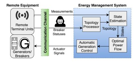
Figure 1.1: A stealthy attack in power grids SCADA network, where an attacker compromises the communication channel to inject malicious data.
