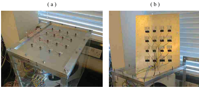
Figure 21. Prototype smart panel with a 4 \times 4 array of decentralized velocity feedback loops formed by square piezoelectric patch actuators with accelerometer sensors at their centers [33].
