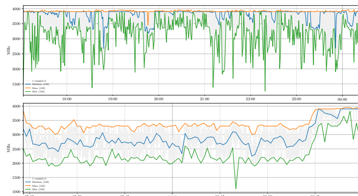
■ Figure 1 Illustration of the CPU frequency scaling when running the sequential solver CaDiCa1 on the considered instance set by solving in parallel 1 instance (upper) and 8 instances (lower).
