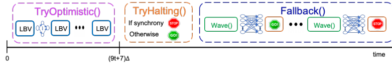
■ Figure 3 Illustration of the optimistic protocol. Both parts form a sequential composition of LBV instances.
