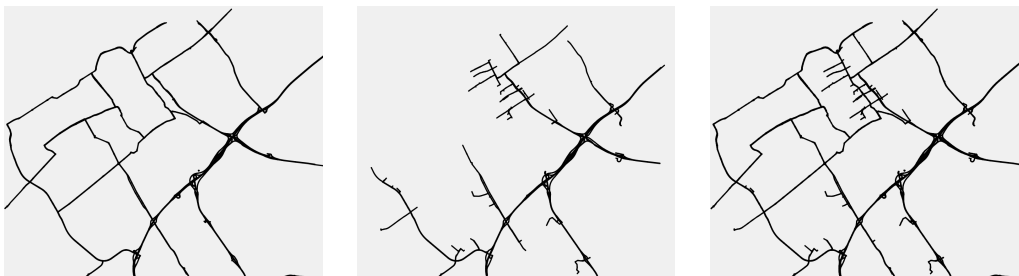
■ Figure 2 Selection by road type (left) and by traffic (middle), combination of both (right).
