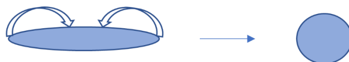
Figure 6. Theoretical example of intraparticle dissolution, where the edges of a needle shaped particle dissolve and recrystallise on other facets of the API particle, changing the particles morphology from needle shape to spherical shape. From an LD perspective, this habitus change would be interpreted as a particle size reduction.
