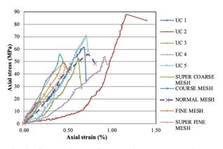
Fig. 4 - Comparison UCT DEM/BPM model with the different mesh size
