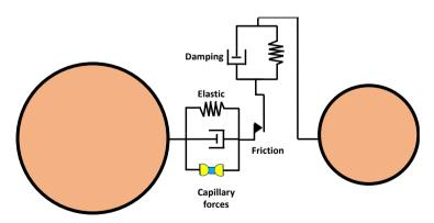
Fig. 1 - Illustration of the bond contact model between particles
