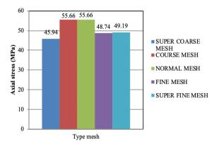
Fig. 5 - Comparison uniaxial compressive strength of different mesh UCT DEM/BPM model
