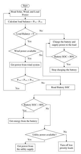
Fig. 2 - Proposed algorithm for load management
