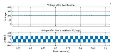
Fig. 11 - Voltage after rectification of WAPDA supply, and load voltage
