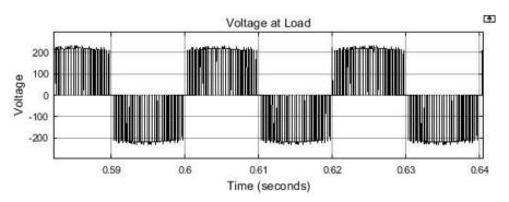
Fig. 7 - Output voltage from the SPWM inverter (close-up view)
