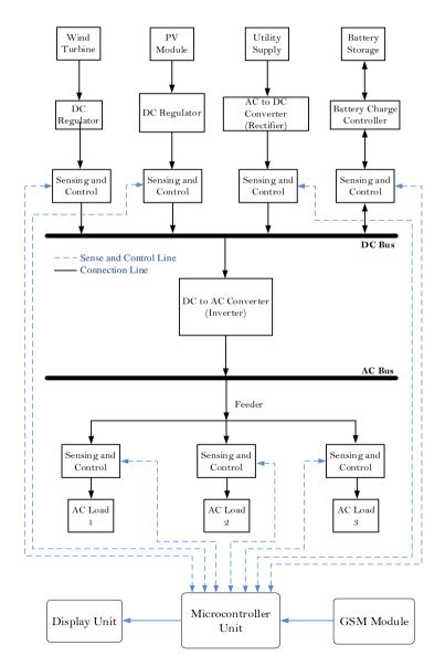
Fig. 3 - The complete model of the system
