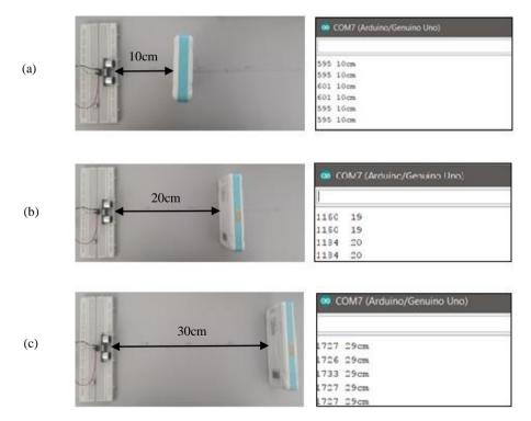
Fig. 8 - Experiment setup (left images) and results (right images) for three cases. The distances between sensor and target at (a) 10 cm, (b) 20 cm and (c) 30 cm
