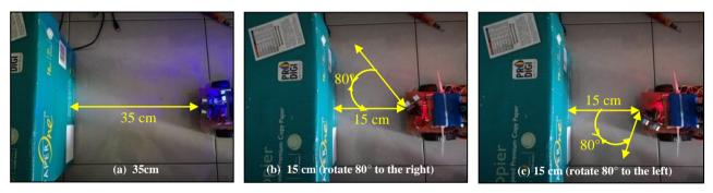
Fig. 11 - Distance between robot and obstacle
