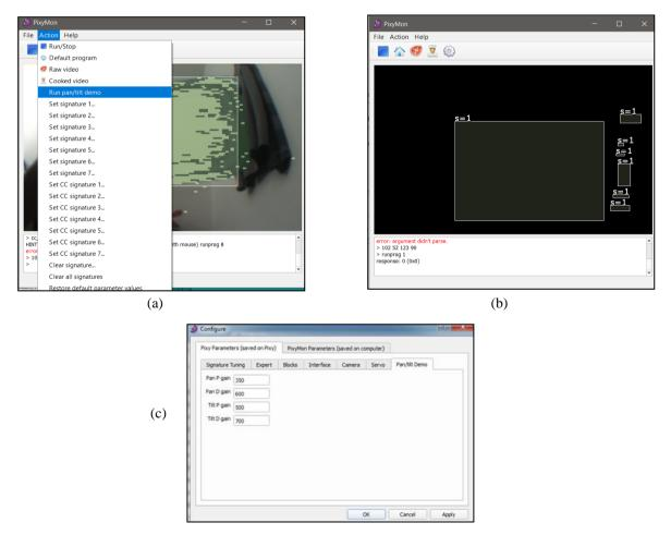
Fig. 10 - (a) Setting a signature; (b) Tracking a signature in Pixy cam; (c) Pan/tilt demo parameters
