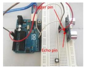
Fig. 7 - Experimntal setup for experiment on ultrasonic sensor
