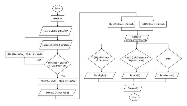
Fig - 4 Flowchart of the algorithm for CREC obstacle avoidance system.
