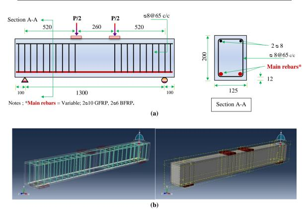
Fig. 4 - The proposed rectangular beams; (a) Layout details (dimensions are mm); (b) Finite element modeling
