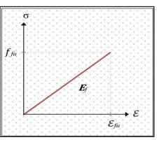
Fig. 8 - Typical linear elastic stressstrain behavior of FRP bars
