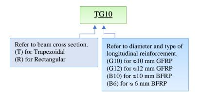
Fig. 1 - Nomenclature of the tested beams
