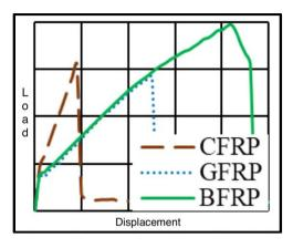
Fig. 13 - Typical load–deflection curve of conventional concrete beams reinforced with different types of FRP bar (carbon, glass, and basalt) FRP based on (Almeida Junior, Parvin) [24]
