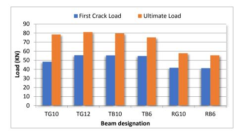
Fig. 11 - The load carrying capacity of all tested beams
