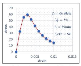
Fig. 5 - Analytical curve for HS-SFRC in compression used in this study
