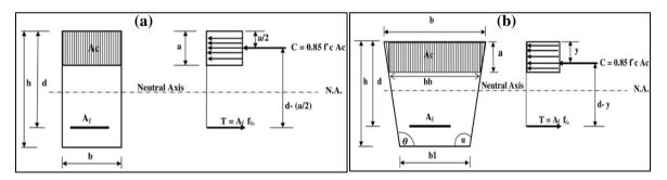
Fig. 17 - Equivalent rectangular flexural stress block distribution of singly FRP reinforced beam cross sections; (a) Rectangular cross-section beam; (b) Trapezoidal cross-section beam
