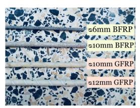
Fig. 10 - The proposed types and diameters of FRP rebars used in this study
