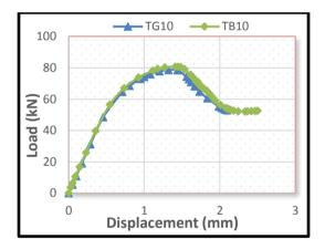
Fig. 14 - Load-deflection curves for beams TG10 and TB10
