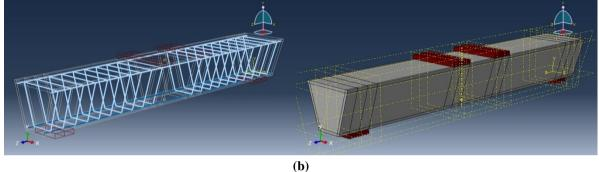
Fig. 3 - The proposed trapezoidal beams; (a) Layout details (dimensions are mm); (b) Finite element modeling
