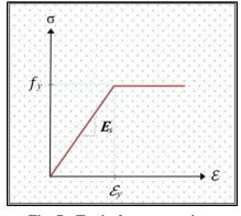
Fig. 7 - Typical stress-strain curve for steel reinforcing bar
