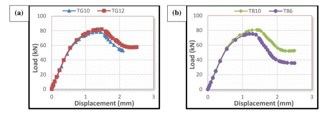
Fig. 15 - Load-deflection curves; (a) Beams TG10 and TG12; (b) Beams TB10 and TB6
