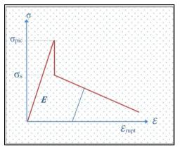
Fig. 6 - Model of tensile behavior in FRC proposed by La Borderie (1991) [17]
