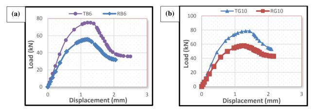
Fig. 16 - Load-deflection curves; (a) Beams TB6 and RB6; (b) Beams TG10 and RG10
