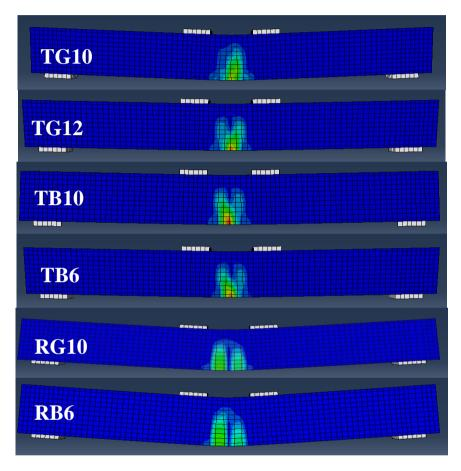
Fig. 18 - Crack patterns at failure of all beams models
