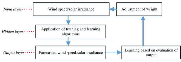
Fig. 7 - Implementation of ANN for forecasting of solar irradiance/wind velocity
