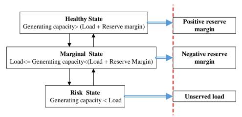
Fig. 8 - System well-being model
