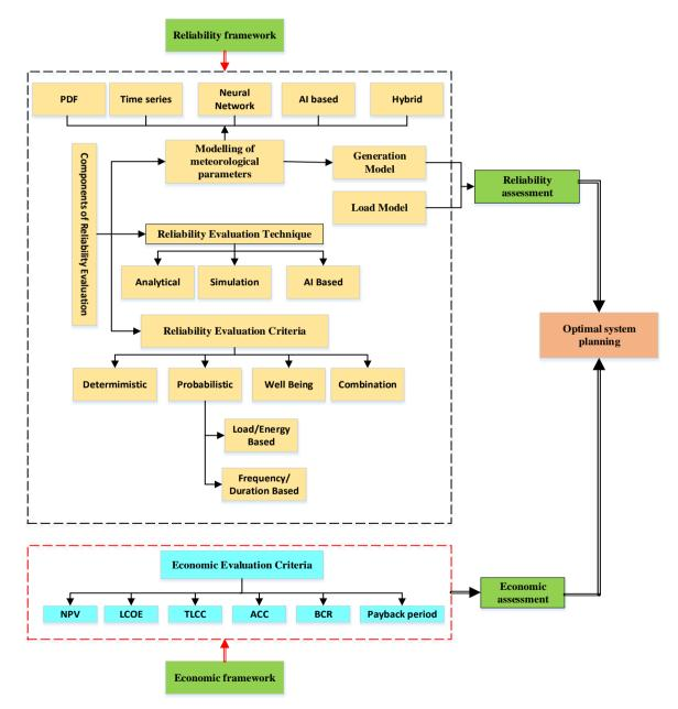
Fig. 2 - Schematic of reliability and economic evaluation framework of HPS
