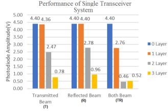
Fig. 3 - Attenuation effects according to the layer of filters applied for cases T, R, and TR in a single transceiver system
