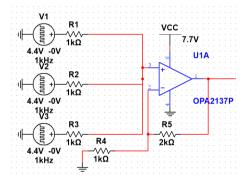
Fig. 4 - Op-Amp configuration for summing amplifier
