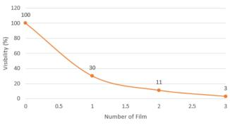
Fig. 1 - Measured visibility of a solar tinted film
