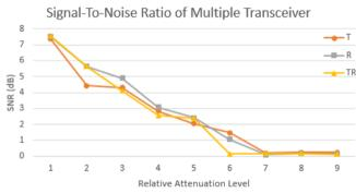
Fig. 12 - Signal-to-noise ratio over attenuation level under the meodeled turbulence
