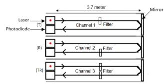
Fig. 2 - Definition of cases of T, R, and TR according to the placement of filter(s) along the laser transmission path
