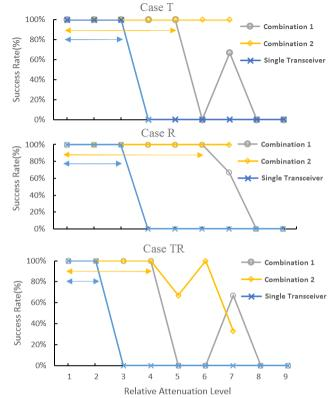
Fig. 14 - Success rate of transmission over relative attenuation level bit
