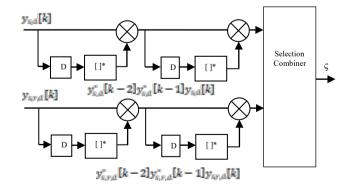
Fig. 2 - The block diagram of SC scheme at the receiver
