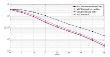
Fig. 3 - Comparison of the BER performance for the conventional MRC, semi MRC, direct combiner and proposed SC scheme based on MSDD when  $\sigma_{\overline{s},r}^2 = 1$ ;  $\sigma_{r,d}^2 = 1$ ;  $\sigma_{\overline{s},d}^2 = 1$  for DDBPSK
