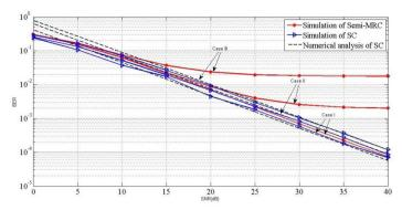
Fig. 7 - Theoretical numerical analysis and simulation BER of the DD-AF system with semi MRC and SC using BPSK under different fading rates and symmetrical channels ( $\sigma_{a,d}^2 = 1$ ;  $\sigma_{a,r}^2 = 10$ ;  $\sigma_{r,d}^2 = 1$ )
