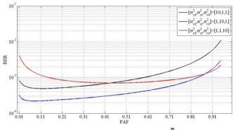
Fig. 5 - Function of BER for PAF at  $\frac{P}{N_0} = 20 \ dB$
