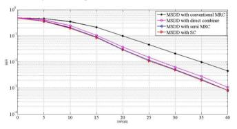
Fig. 4 - Comparison of the BER performance for the conventional MRC, semi MRC, direct combiner and proposed SC scheme based on MSDD when  $\sigma_{s,r}^2 = 1$ ;  $\sigma_{r,d}^2 = 1$ ;  $\sigma_{s,d}^2 = 1$  for DDQPSK
