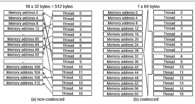
Fig.2 - This figure shows the Coalescing process
