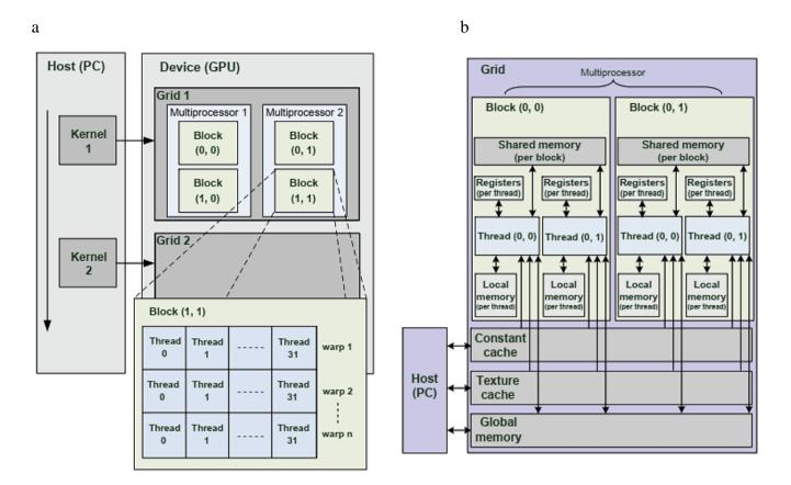
Fig 1 - (a) CUDA hierarchy of Grids, threads and blocks (b) CUDA Memory Hierarchy
